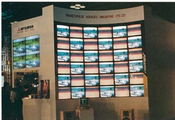
The 6 x 6 Laserpoint Pixelite videowall with 2 x 2 projection wall to left.
